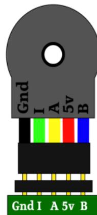
Figure 21. Encoder Pinout
