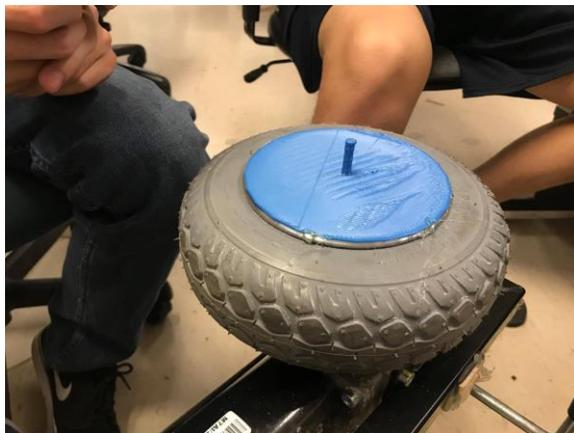
Figure 30. Encoder Adapter Mounted
